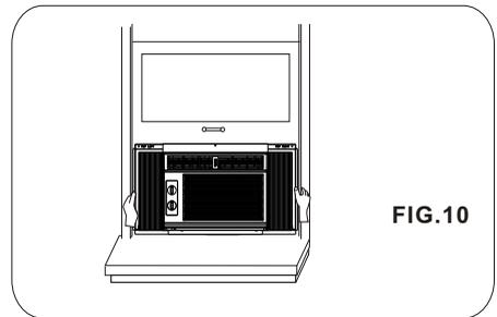
When the air conditioner is properly installed, it should tilt slightly down at the back. If it is set correctly in the window, it will hang lower in the back automatically. If it does not, there is a problem with the installation.
